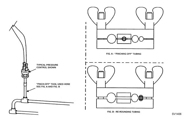
Figure 7-10. Using Pinch-Off Tool
